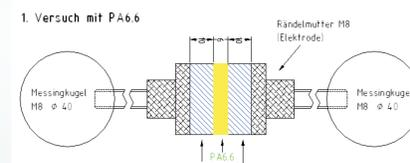
**problems:** the knurled nuts are not adaptive as electrodes
