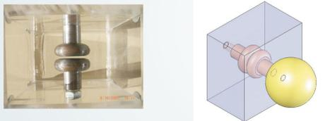
**problems:** - homogeneous field requires very high voltages to receive measured values
