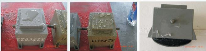
test item without coating      test item with coating      coating peels off
