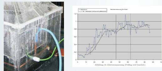
constant bedewing is needed, while the test item has to deal with high voltages
